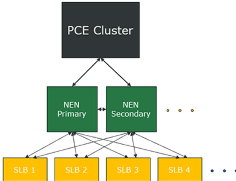
A PCE cluster supports multiple NENs per PCE, which can consist of multiple single node NENs, multiple NEN HA pairs, or a combination of both.
