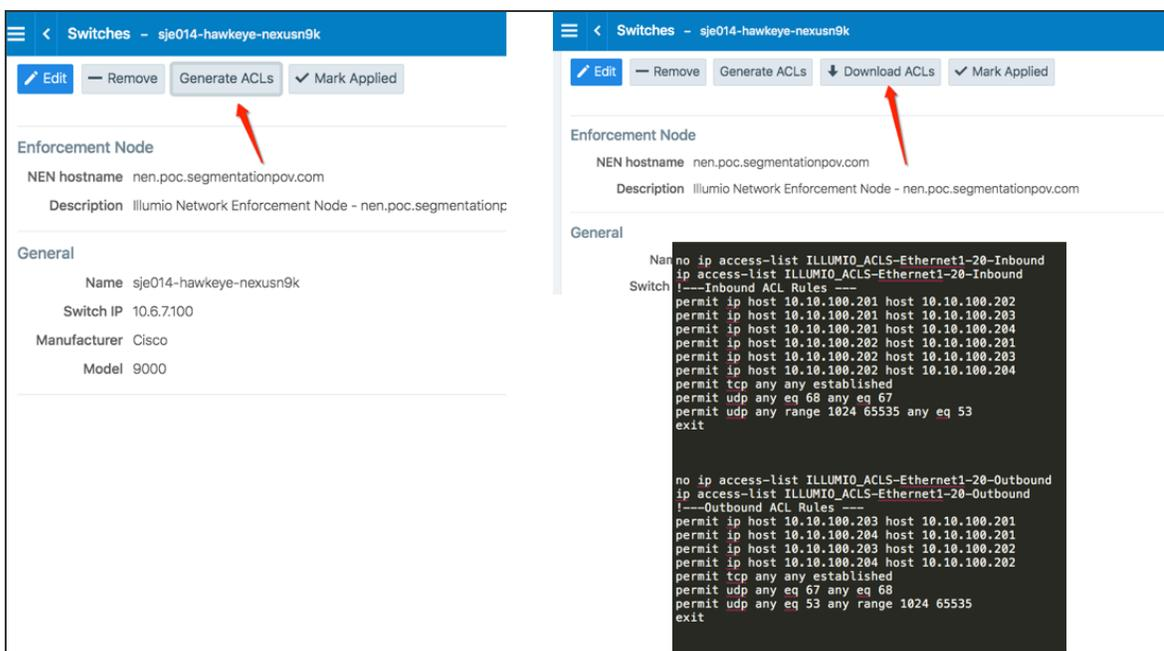
The workloads associated with the switch remain in an **Active (Syncing)** policy sync state until you click the **Mark Applied** button on the Switches page.
