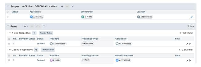
The following example shows a better way to write the extra-scope rule because it restricts inbound traffic from the R-SNAP role, the A-SYSTEMS application, and the E-PROD environment in all locations.
