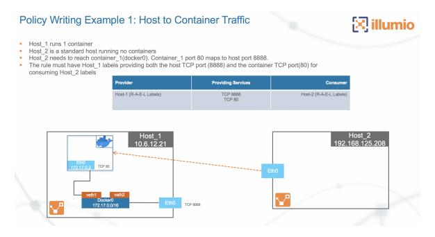
To allow access to container on Host\_1 port 80, create an intra-scope rule for access within the application group and extra-scope rule for access from outside of the application group.
