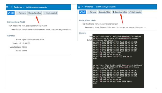
The workloads associated with the switch remain in an **Active (Syncing)** policy sync state until you click the **Mark Applied** button on the Switches page.
